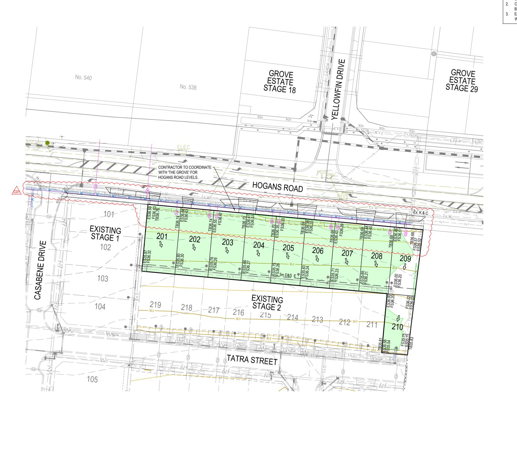
**NOTES** CONTRACTOR TO DELAY CONSTRUCTION OF CROSSOVERS AND PARKING BAYS ALONG HOGANS ROAD UNTIL KERBS AND CHANNELS HAS BEEN CONSTRUCTED.
